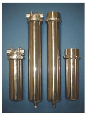
All types are produced according pressure device guideline 97/23/EG article 3 § 3 'Gute Ingenieur-spraxis'. The housings can be operated with liquids that belong to the group 2 (article 3), if a vapour pressure of 0,5 bar is not exceeded.
